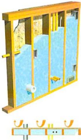
STYROFOAM™ SPF Insulation provides an edge-to-edge air seal, effectively blocking random air leakage and moisture intrusion.
