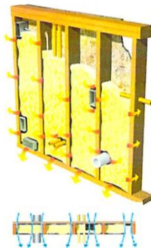
Air escapes easily through and around fibrous batt insulation, decreasing insulation efficiency and trapping dirt and moisture in the fibers.
